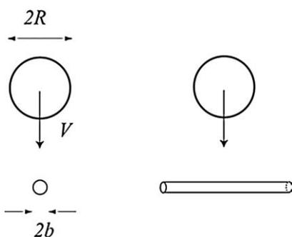
Fig. 6. Sketch of the experiment: a drop of radius  $R$  falls on a horizontal fiber of radius  $b$ .
