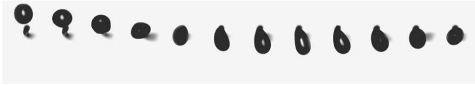
Fig. 7. Set of pictures taken each 4 ms (front view, as sketched in Fig. 6a). The drop of silicon oil ( $\eta = 5$  m/s) falling at 20 cm/s is entirely captured by the fiber.
