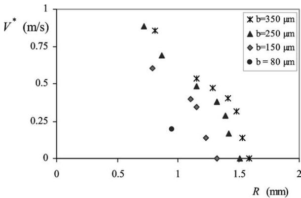
Fig. 9. Critical velocity for crossing a fiber of radius  $b$ , as a function of the radius of the impacting drop  $R$ . The drops consist of water, and the fibers of nylon.
