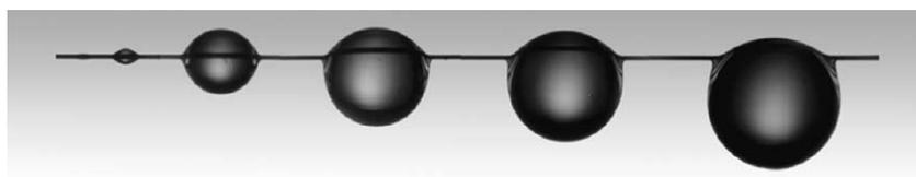
Fig. 1. Drops of silicon oil of various volumes ( $\Omega = 0.01, 0.10, 0.23, 0.32$ , and  $0.52 \text{ mm}^3$ , from left to right) hanging from a horizontal fiber of radius  $b = 12 \mu\text{m}$ .
