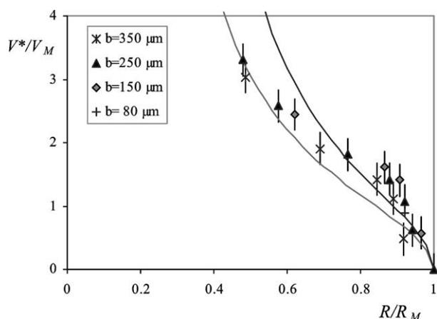
Fig. 11.  $V^*/V_M$  as a function of  $R/R_M$  for different fiber radii;  $R_M$  and  $V_M$  are defined in Eqs. (2) and (5). The experimental data collapse onto the same curve, which is quite well fitted by Eq. (7), drawn in full line for two fiber radii ( $b = 150 \mu\text{m}$ , in gray, and  $b = 350 \mu\text{m}$ , in black).
