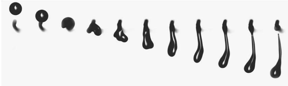
Fig. 8. A drop of silicon oil ( $\eta = 5$  mPa s) impacting at  $V = 95$  cm/s a horizontal fiber of radius  $b = 350$   $\mu\text{m}$  is not trapped by the solid. An elongated drop forms below the fiber and eventually detaches, and only a small amount of liquid remains captured. Interval between successive pictures 2 ms.
