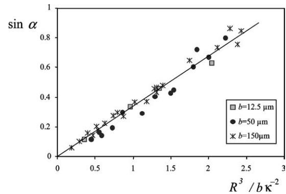
Fig. 5. Sine of the angle  $\alpha$  (see Fig. 4 for the definition of  $\alpha$ ) as a function of  $R^3/b\kappa^{-2}$ ,  $R$  being the drop size,  $b$  the fiber radius, and  $\kappa^{-1}$  the capillary length.
