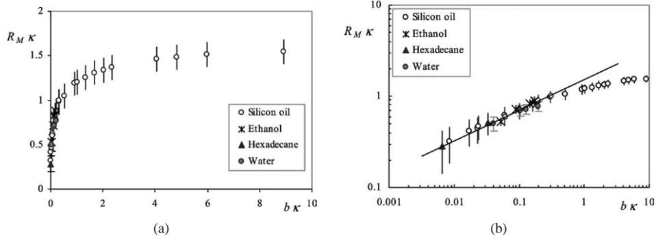
Fig. 3. Radius  $R_M$  of the largest drop hanging on a fiber, as a function of the fiber radius  $b$ . Both quantities are normalized by the capillary length  $\kappa^{-1}$  and are drawn in normal coordinates (a) or in logarithmic ones (b).
