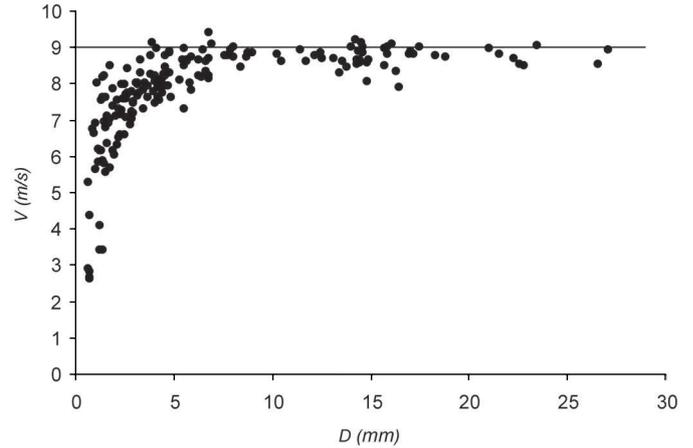
Fig. 2: Terminal velocity  $V$  of a water drop falling in air, as a function of its equatorial diameter  $D$ . For drops smaller than the capillary length, the velocity quickly increases with the size (eq. (1)). For larger drops, which are flattened (fig. 1a), the velocity saturates (eq. (4)).
