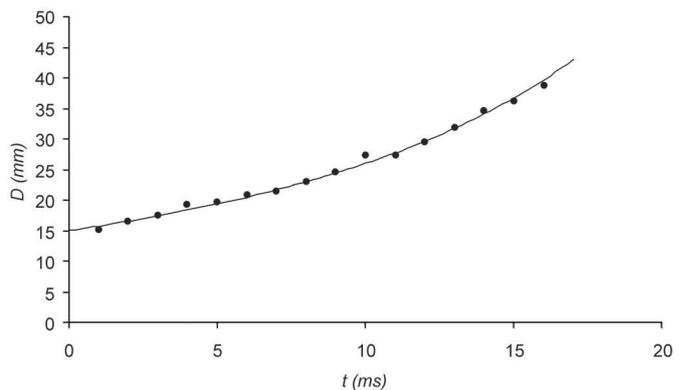
Fig. 4: Inflation of a bag-shaped drop: the bag diameter is plotted as a function of time. The non-linear growth is observed to be well fitted by eq. (5), drawn in full line with  $\alpha = (6/\pi)^{1/2}$  (the value expected for an isotropic growth) and  $m = 0.94$  g, in fair agreement with the mass unprecisely deduced from the bag-shaped drop ( $m = 1.0 \pm 0.7$  g).
