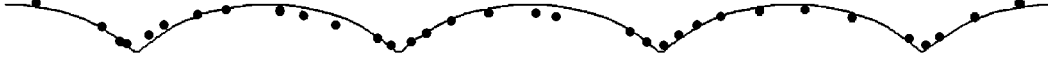
Fig. 3. – Trajectory of a track (a bubble of size 100 \mu\text{m} ) placed just below the surface of a glycerol drop of radius R = 1.6 \text{ mm} running down a super-hydrophobic plate. The points are the data deduced from a film (error bar of order the point size). The line is a cycloid of equation: x = t + 0.75 \sin t , y = 0.75 \cdot 0.73 \cos t , where the coefficients 0.75 and 0.73, respectively take into account the position of the track inside the drop and the eccentricity of the drop ( \varepsilon = 1.3 ) due to gravity.
