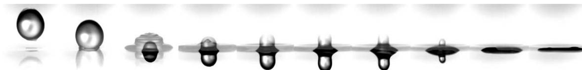
Fig. 2. Set of pictures taken each 2 ms ( $D = 3.5$  mm,  $r = 390$   $\mu\text{m}$ ,  $V = 50$  cm/s). The drop (silicone oil of surface tension  $\gamma = 16$  mN/m and viscosity  $\eta = 0.5$  mPa s) is entirely captured by the surface. The hole is in the middle of each frame. Below it, a liquid finger transiently forms and retracts; above it, we see in the pictures both the impacting drop and the reflection of the finger.
