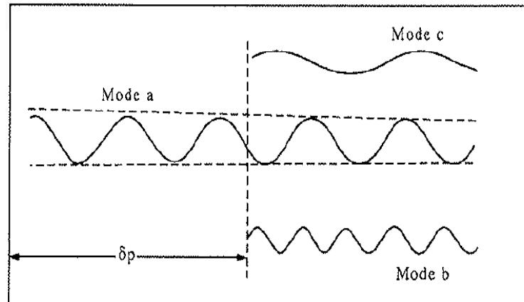
Fig. 8. From the distance  $\delta p$ , mode conversion appears at the second order.
