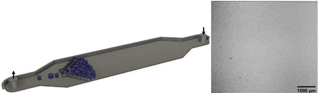
Figure 1: A) Schematic overview of the hopper flow experiment. The hydrogel particles (blue) are forced through the constriction by imposing a flow. B) Example of an experimental packing of 120-160  $\mu\text{m}$  particles.
