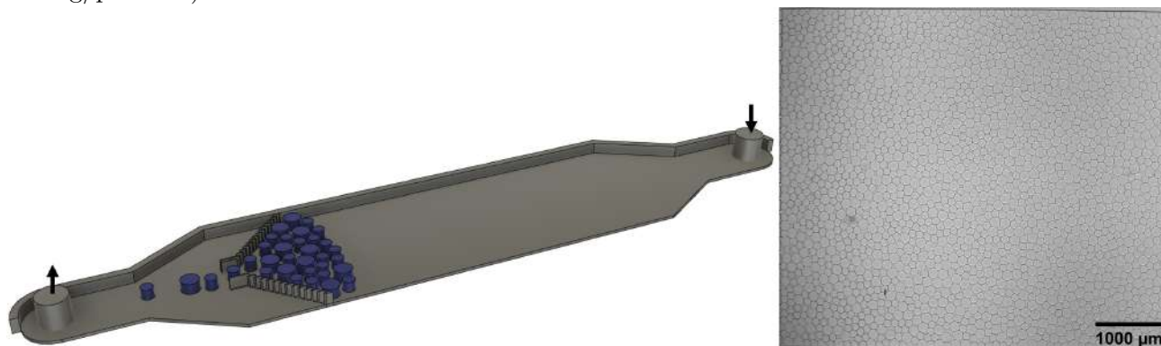
Figure 1: A) Schematic overview of the hopper flow experiment. The hydrogel particles (blue) are forced through the constriction by imposing a flow. B) Example of an experimental packing of 120-160 \mu\text{m} particles.
